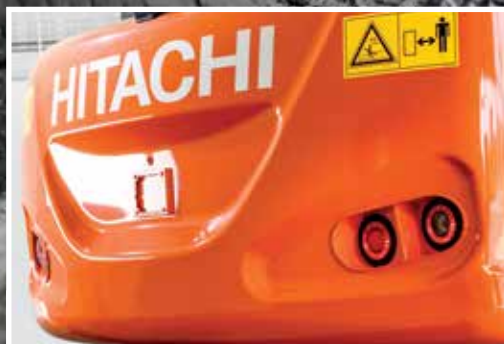
LED tail lights are easily maintained.
