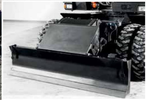
Large blade cylinder cover offers greater protection.
