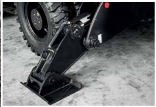
Reliability is enhanced by a reinforced outrigger cylinder cover.
