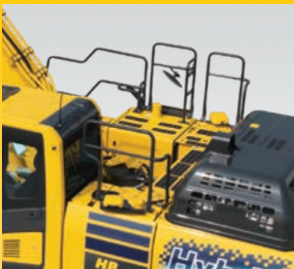
Hand rails and anti-slip plates
